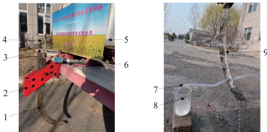
b. 叶脉状内通道深松铲整机装置 c. 叶脉状内通道分支出口流速测量装置 b. Leaf vein shaped inner channel deep loosening shovel c. Flow velocity measurement device for branch outlet of leaf vein shaped internal channel
