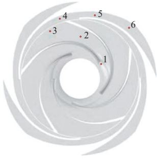
注：1~3 为首级叶轮压力脉动监测点；4~6 为首级导叶压力脉动监测点。 Note: 1-3 are the first impeller pressure pulsation monitoring point; 4-6 are the first-stage guide vane pressure pulsation monitoring point.
