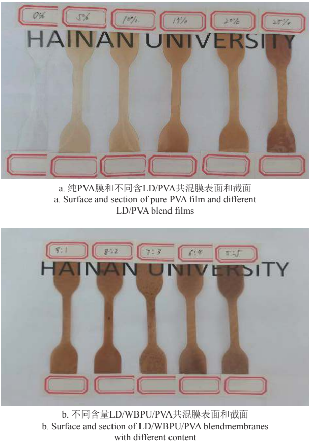
图 3 制成的不同共混膜样品透光情况 Fig.3 Light transmission of different blended film samples
