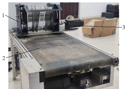
1.取苗装置 2.带式输送机 3.调速电机 1.Seedling-taking device 2.Belt conveyor 3.Adjustable speed motor
