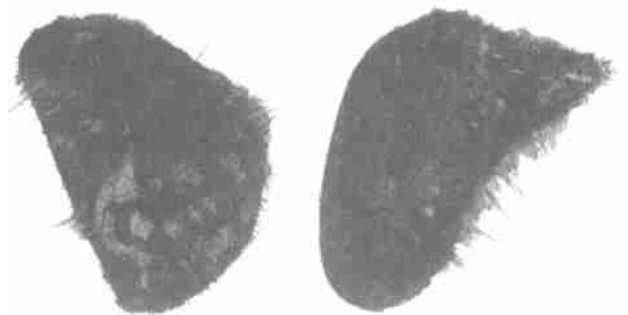
图 16 牛蹄角三维曲面与原始点群的误差分析针状图 Fig. 16 Error map in needle between cattle hoof exterior configuration model and original points
